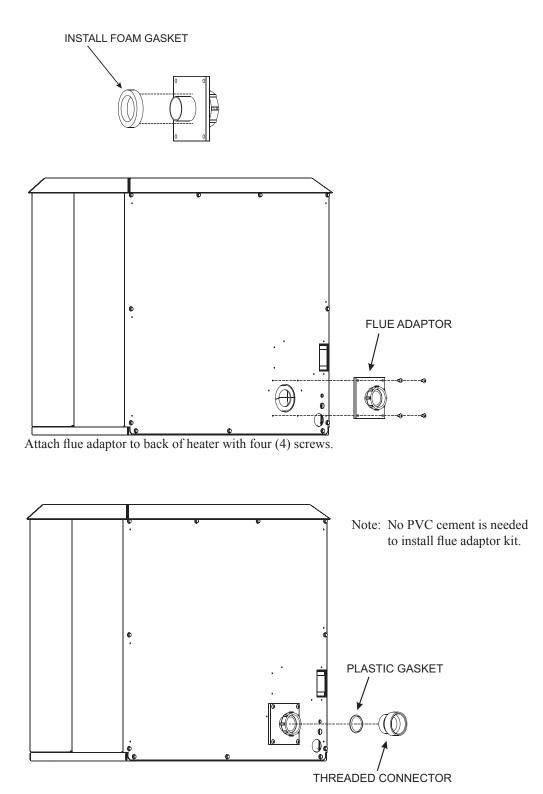
Install plastic gasket and screw threaded connector to the flue adaptor. When these connections are made, continue with your vent run. Cement all PVC joints on vent run.
